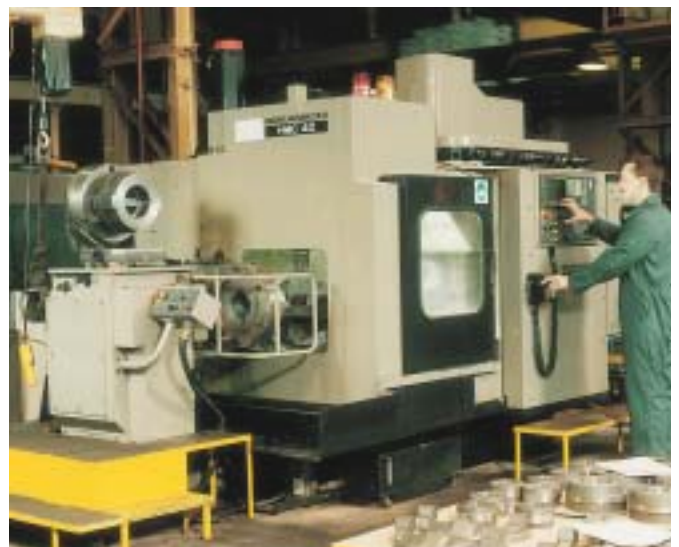
Four pallet CNC machining centre with auto tool changer
