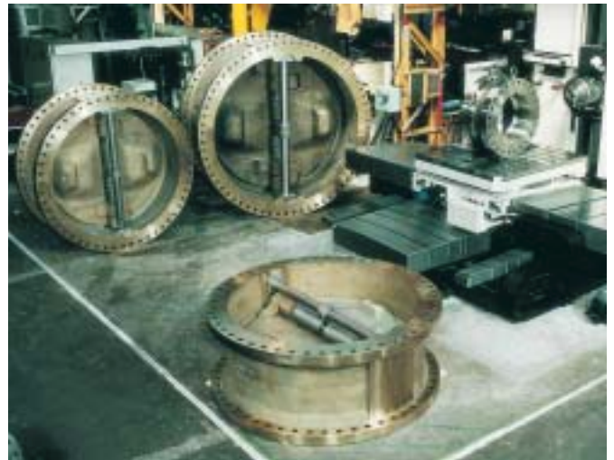
Two 66" 150 lb and one 84" 150 lb Check Valves in Aluminium Bronze
