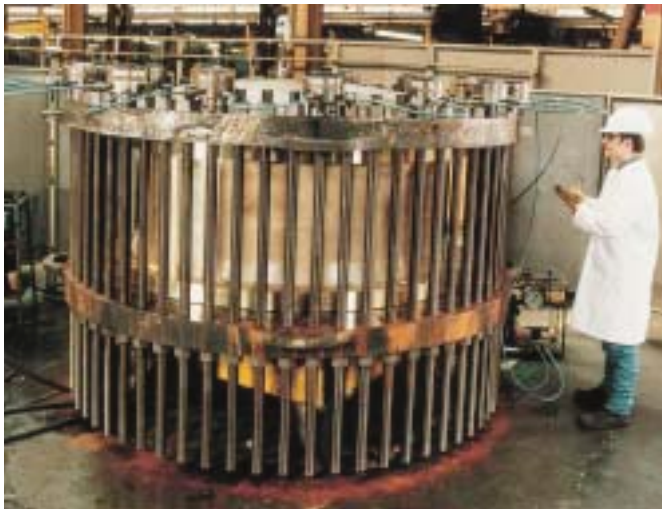
84" 150 lb valve undergoing hydrotest in Goodwin factory
