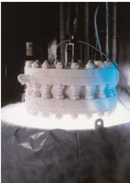
24"ANSI 150lb Check Valve on Cryogenic Test
