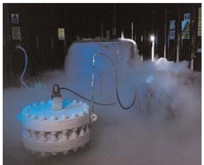
Cryogenic test facility for helium leak testing
