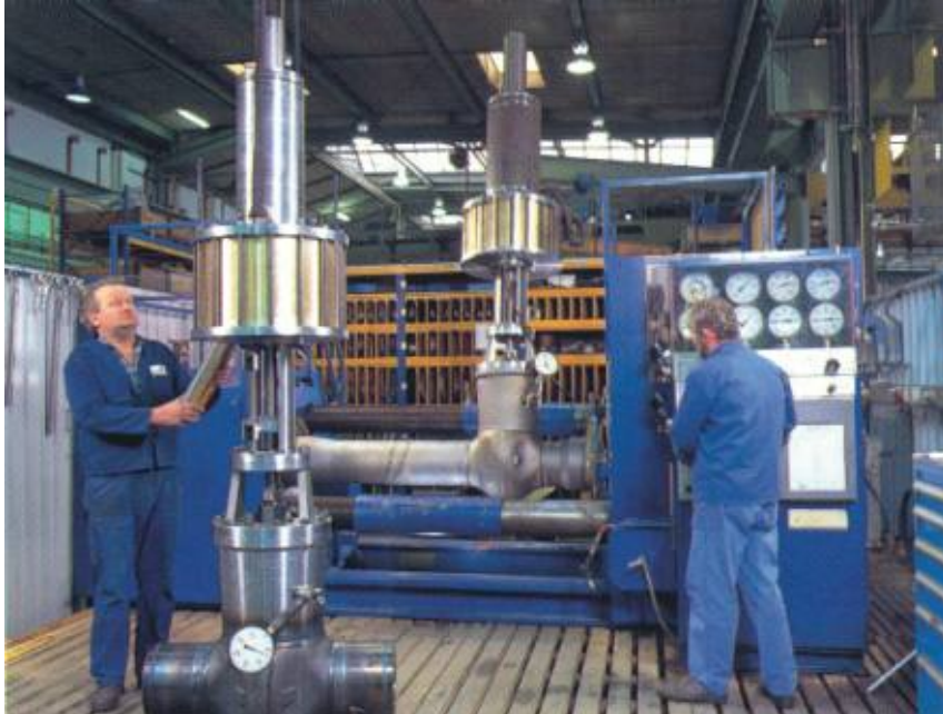
DN 300/250 PN 63 Gate valve with pneumatic Actuator under testing
